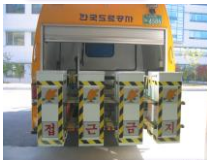
2D antenna array for 3D surveys
