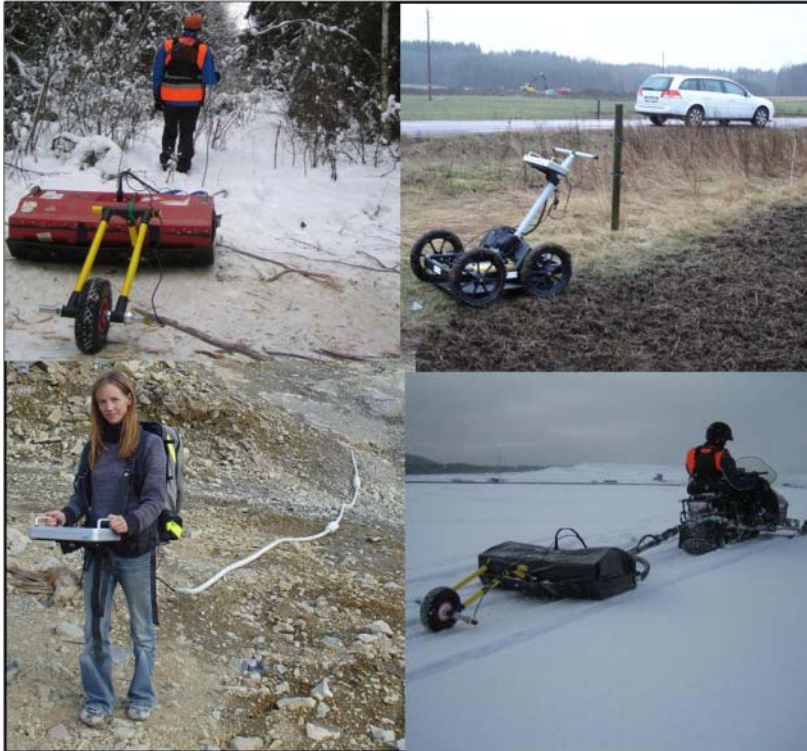
Figure 5. Typical GPR systems for site investigations
